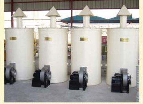
Carbon Filter Tanks for Environmental System to Generate fresh air
